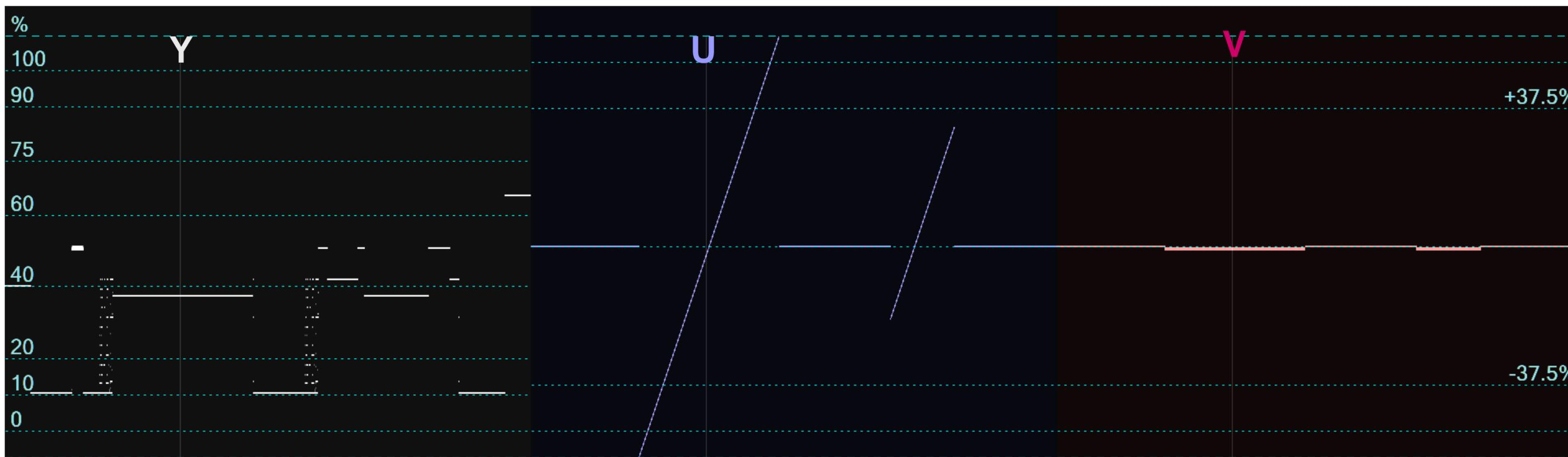
VQCSE Main Palette YUV data are **correct** – Y and V values are **constant** within the selected area (waveform horizontal lines);
