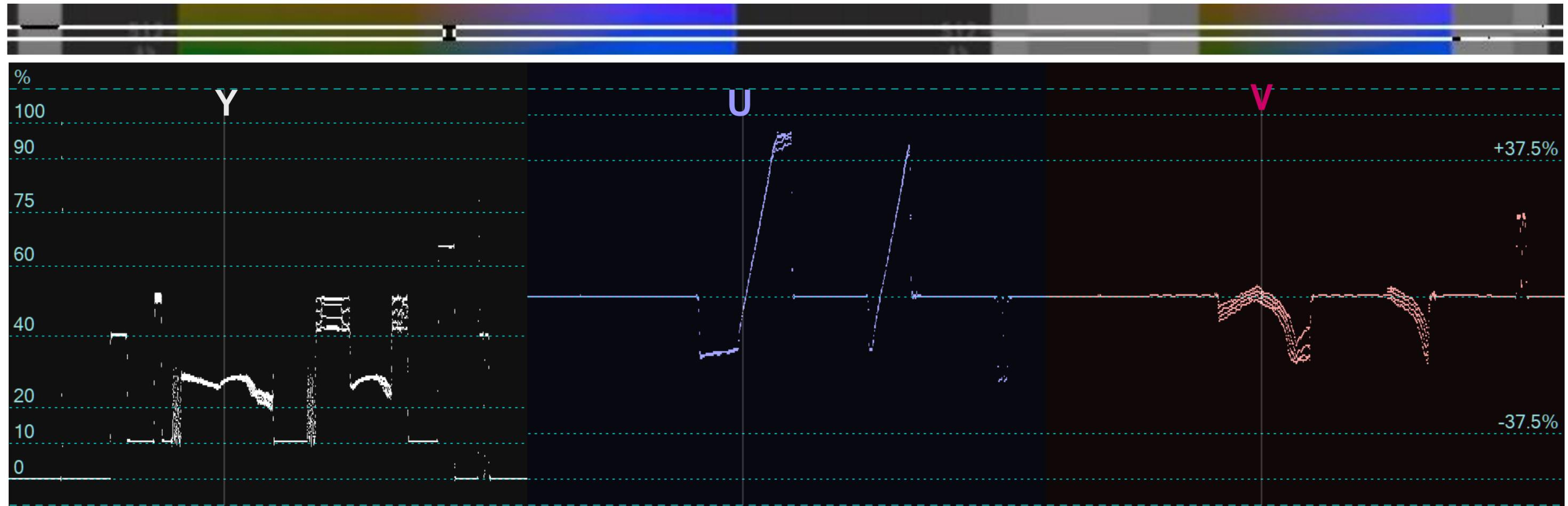
Palette SDR YUV data are **seriously distorted** – within the **Valid YUV Range** Y and V waveforms are **visibly bent**;
