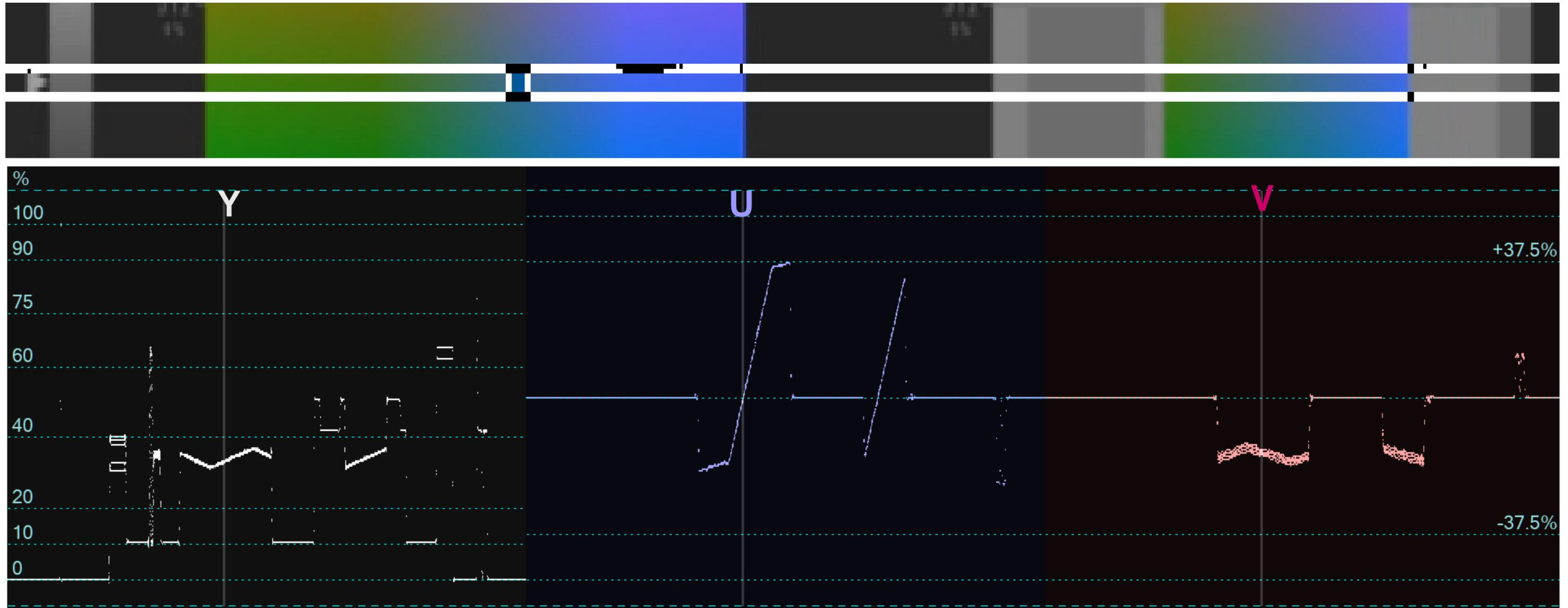
Palette YUV data are **not exactly correct** – Y and V values are **not perfectly flat** or **linear ramps** within **Valid YUV Range**;
